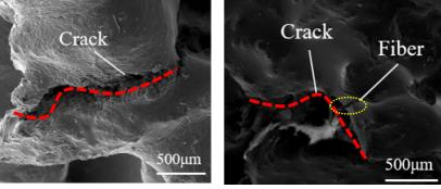
□ The microscopic pictures show that the fiber plays a certain tensile role when the asphalt mixture is damaged by force.
